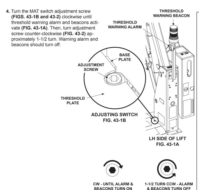
**5.** Step on threshold plate. Warning alarm and beacons should activate. If the warning alarm and beacons do not activate, slightly turn adjustment screw (FIGS. 43-1B and 43-2) clockwise. Repeat until warning alarm and beacons activate when stepping on threshold plate and deactivate stepping off threshold plate.
